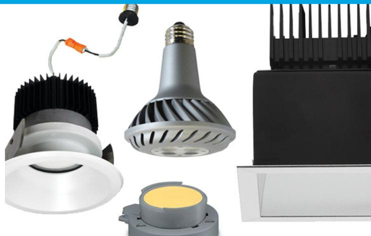
**Clockwise from left: an LED downlight retrofit unit, an LED PAR replacement lamp, an integrated LED downlight luminaire, and an LED module.** These four form factors are all used in LED downlights; although none is inherently superior, they each have unique characteristics that can be advantageous in certain applications. This fact sheet focuses on luminaires and retrofit units.
