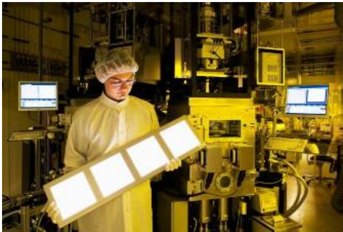
Large Area OLED lighting panel (80x20 cm 2 ) by Fraunhofer IPMS
