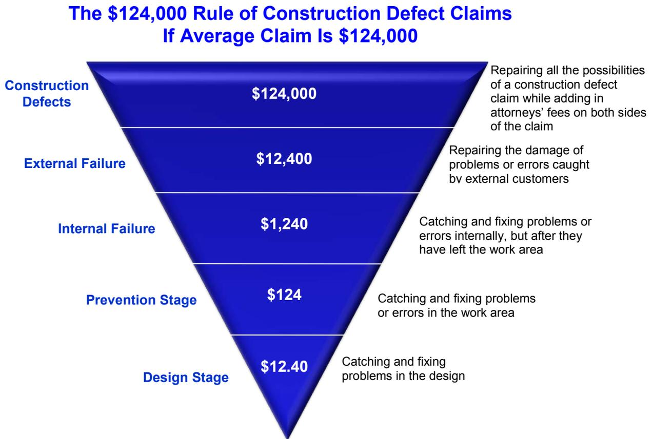
**Figure 4. The construction defect cost triangle**
