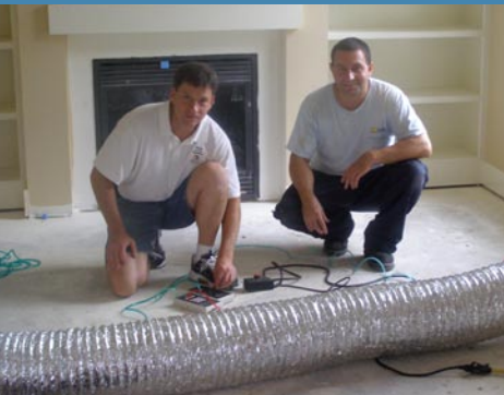
Brian Shaner of Horizon Mechanical and Armin Rudd of BSC performing the duct blast/blower door testing in the Molly Cottage.
