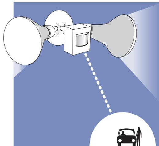
**Motion sensors** automatically turn outdoor lights on when they are needed (when motion is detected) and turn them off a short while later. They are very useful for outdoor security and utility lighting provided by incandescent lamps.
